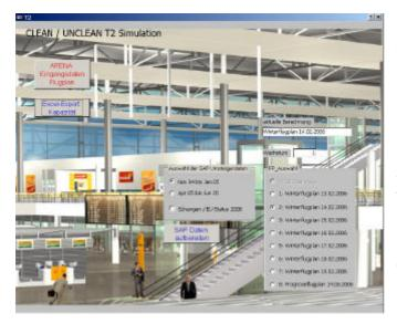
Because of the need to link different data, e.g. the scenario flight schedules and an airport database with information about the EU-status of the airports, we used MS-Access and VBA to pre-process the input-data for ARENA. A user interface allowed easily to set the required parameters for the simulation. The transfer passenger flows between arrival and departure flights were calculated using a 3-step VBA algorithm.
